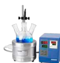
Temp. Control and safety protection
