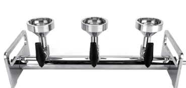
3-Branch stainless steel manifold BioVac330 Order No.: 167103-23
