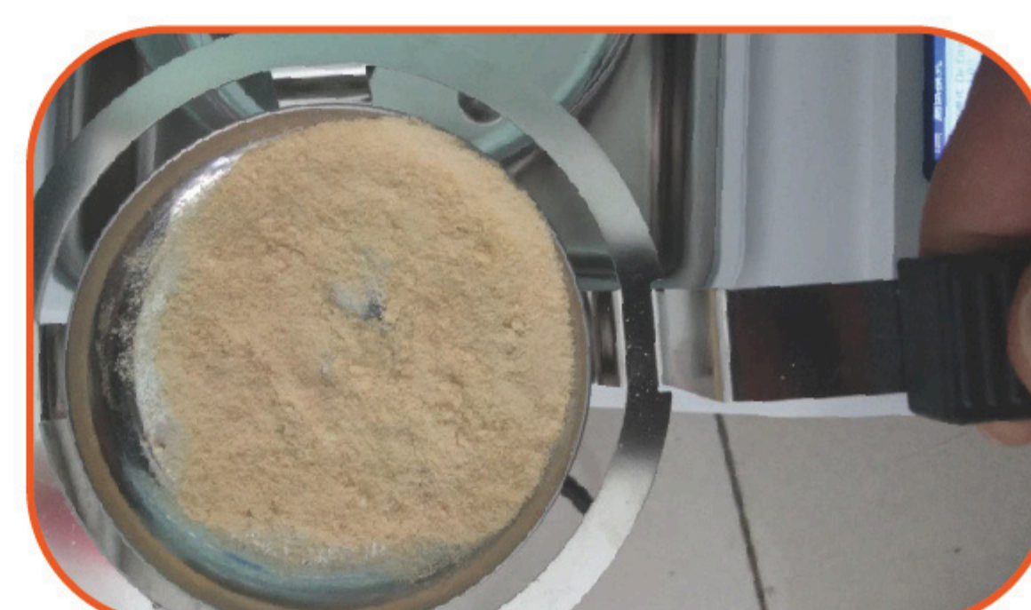
Humanized design sample plate handle heat insulation treatment
